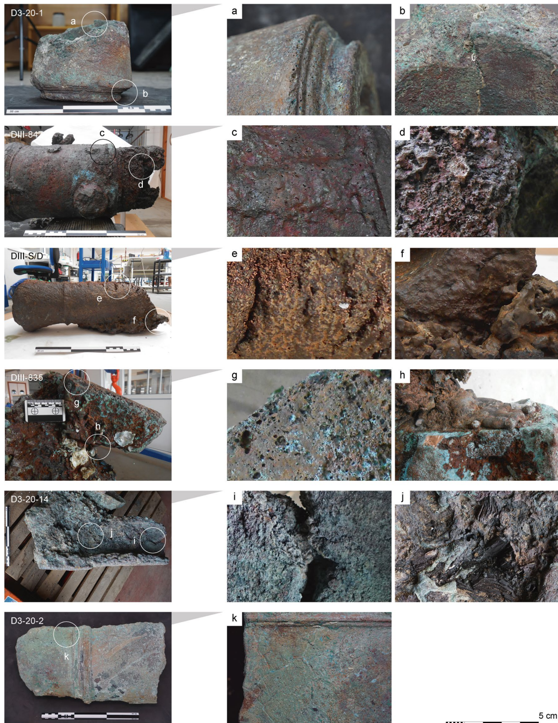
Fig. 7 A detailed view of macroscopic casting defects in a selection of pieces: a gas porosity: pinholes; b cracks: cold tear; c vitrification; d sponginess; e open shrinkage cavities or pipes; f mould collapse; g
